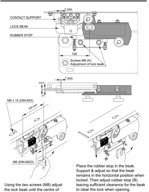
the pivot pin is 100 mm from the leading edge of the hanger.
